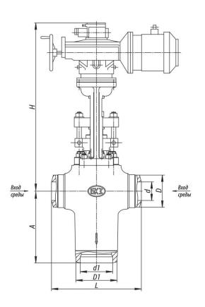
Pipeline connection: welded connection.
